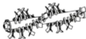
ROTOR HELICOIDAL "HELICOCUT"
